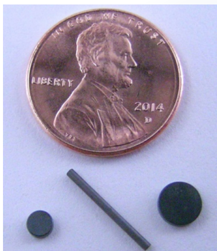
Figure 1. SiC temperature monitors available for use in irradiation testing include small rods and disks.
