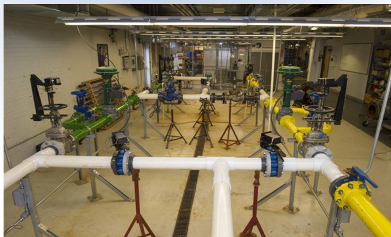
Figure 2: Wireless VPI sensor technology installed at ISU's ESTEC experimental flow-loop.
